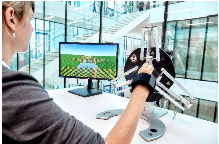
Figure 5: Experimental setup with Delta.3 robot (Force Dimension, Switzerland).
