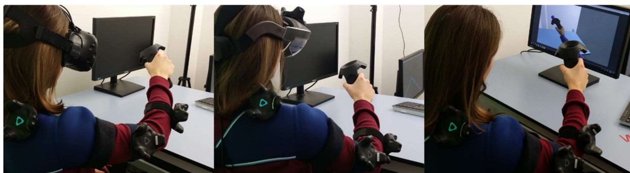
Figure 2: Display modalities. Left: Immersive virtual reality (IVR). Middle: Augmented reality (AR). Right: 2D Screen. In all modalities, participants hold a controller and wear three trackers placed on the shoulder, the upper arm, and the lower arm. In AR, a fourth tracker was attached to the HMD.
